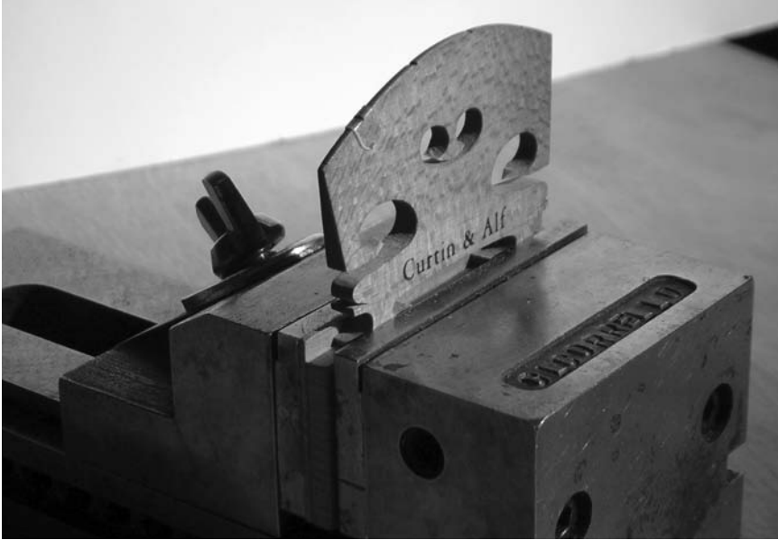
Figure 2. The bridge is held in the jaws of a machinist's vise. A wooden wedge along one jaw complements the taper of the bridge. A wood strip glued to the wedge a few millimeters below the top face of the jaw ensures that the bridge is always clamped at the same distance from the bottom of its foot.
