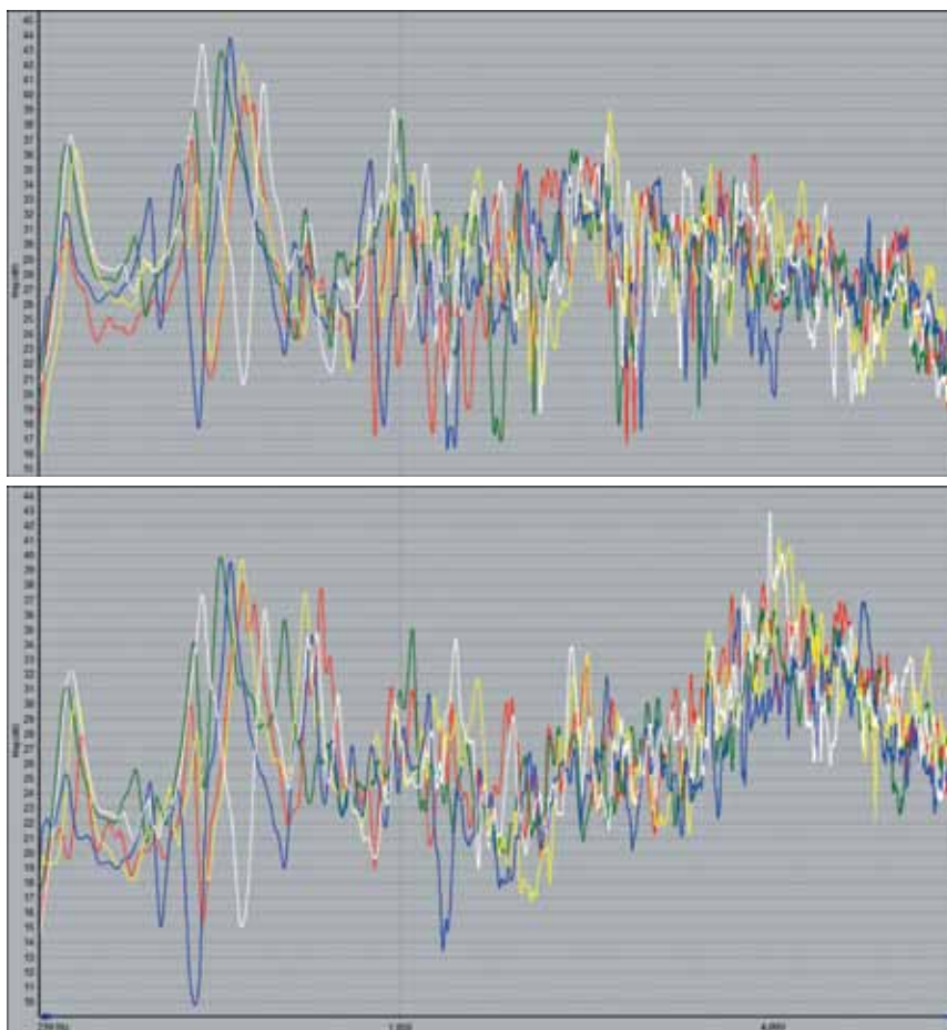
FIGURE 2 Horizontal (top) and vertical (bottom) spectra for the 'Vieuxtemps' (white), 'Jarnowich' (yellow), Guadagnini (green), 'Cathedral' (red) and 'Nachez' (blue). Each line represents the real average of twelve microphone positions, evenly spaced around the instrument, in plane with the bridge, 20cm from the instrument's central axis. Vertical scale: relative amplitude in decibels. Horizontal scale: logarithmic frequency, 250Hz-8,000Hz.
